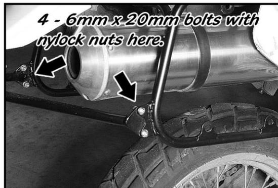
10. Once all of the hardware is in place, please tighten the four bolts on the right rack first, then the four bolts on the left rack and then the four bolts that hold the crossbar in place.
